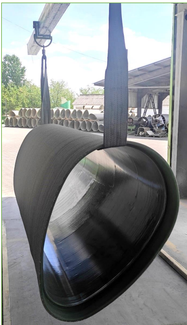
Figure 1: Moving GRP pipes with crane
