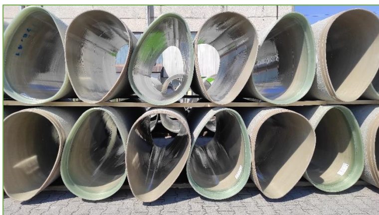
Figure 5: Storage of pipes on wooden bearers
