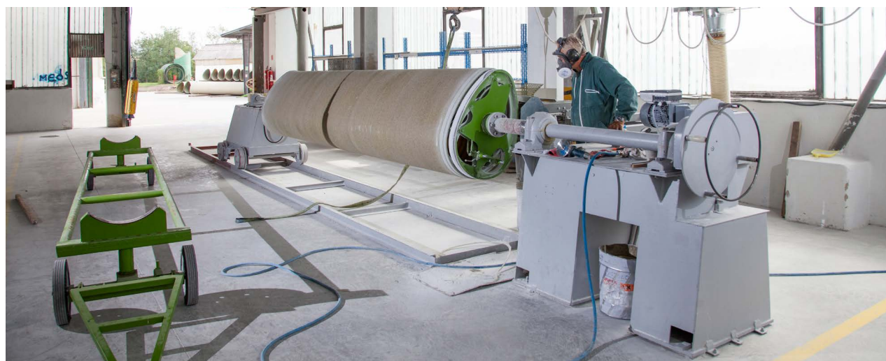
Pipes being cut to size and chizelled
