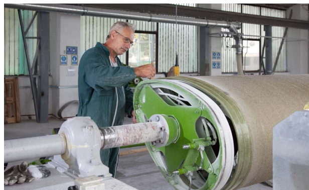
Creating the pipe ends to be connected
